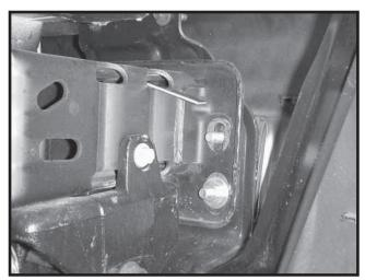
4. Insert correct side pull pod on side where bumper bolts were removed. Put two 1/2" x 1-3/4" bolts through out side edge of pod. In the back where bottom bolt comes through, use 1/2" flat washer, 1/2" lock washer, and 1/2" hex nut. Before tightening bolt, lift bumper up and center top bolt in middle of slot while holding pull pod straight. Put 1/2" flat washer, 1/2" lock washer, and 1/2" hex nut on top bolt and tighten. NOTE: We recommend using "LOCTITE. Blue" on all bolts
